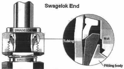
Cross-Section of Swagelok End connection
